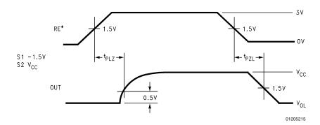
FIGURE 15. Receiver Enable and Disable Waveforms ( $t_{\text{PLZ}},\,t_{\text{PZL}}$ )
