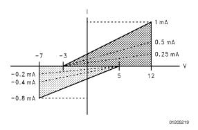
FIGURE 18. Input Current vs Input Voltage Operating Range
