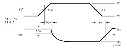
FIGURE 16. Receiver Enable and Disable Waveforms ( $t_{\text{PHZ}},\,t_{\text{PZH}}$ )
