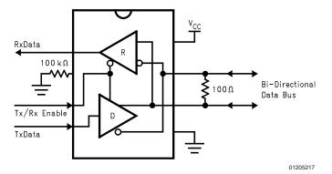
FIGURE 17. Typical Pin Connection
