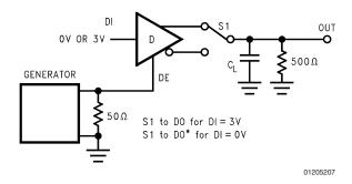
FIGURE 7. TRI-STATE Test Circuit ( $t_{PZH}$ ,  $t_{PHZ}$ )
