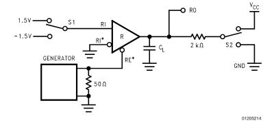
FIGURE 14. Receiver TRI-STATE Test Circuit
