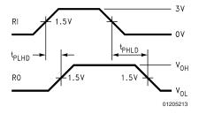
FIGURE 13. Receiver Differential Propagation Delay Waveforms
