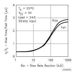
FIGURE 19. Slew Rate Resistor vs Rise/Fall Time
