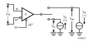
FIGURE 11. Receiver  $\rm V_{OH}$  and  $\rm V_{OL}$
