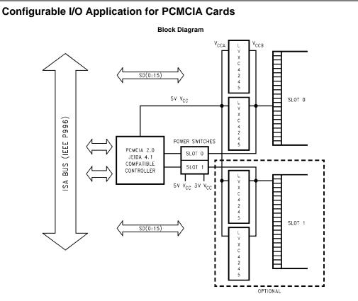
The LVXC4245 is a 24-pin dual supply device well suited for PCMCIA configurable I/O applications. Ideal for low power notebook designs, the LVXC4245 consumes less than 1 mW of quiescent power in all modes of operation. The LVXC4245 meets all PCMCIA I/O voltage requirements at 5V and 3.3V operation. By tying V<sub>CCB</sub> of the LVXC4245 to the card voltage supply, the PCMCIA card
