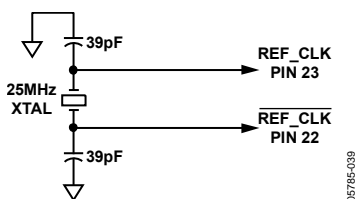
Figure 40. Crystal Configuration for Reference Clock Source
