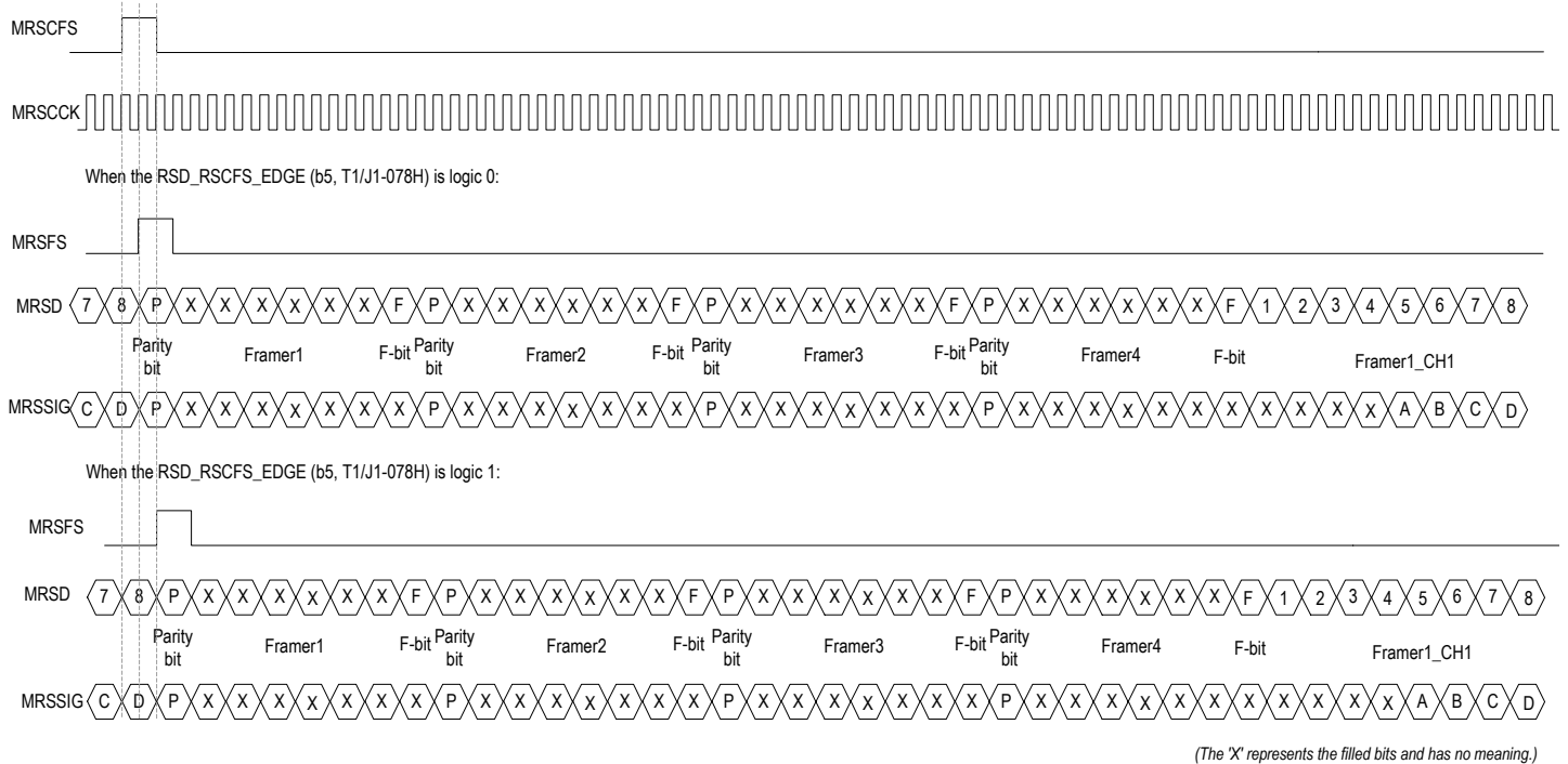
Figure 34. T1/J1 Receive Multiplexed Mode - Functional Timing Example 2
