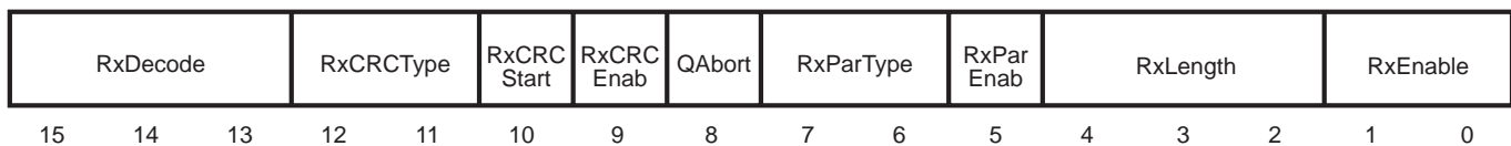
Figure 5-6. The Receive Mode Register (RMR)
