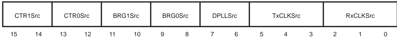
Figure 4-2. The Clock Mode Control Register (CMCR)
