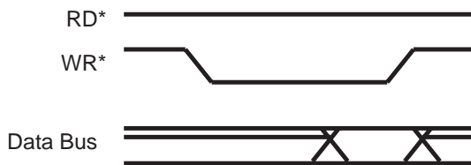
Figure 2-4. /RD and /WR Signaling
