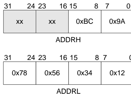
Figure 4.2 Example ADDRL, ADDRH Address Ordering
