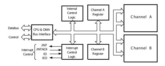
Figure 1. Z85233 Functional Block Diagram
