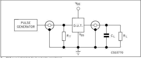
$\begin{array}{l} C_L = 50 p F \mbox{ or equivalent (includes jig and probe capacitance)} \\ R_L = 200 K \Omega \\ R_T = Z_{OUT} \mbox{ of pulse generator (typically 50 \Omega)} \end{array}$
