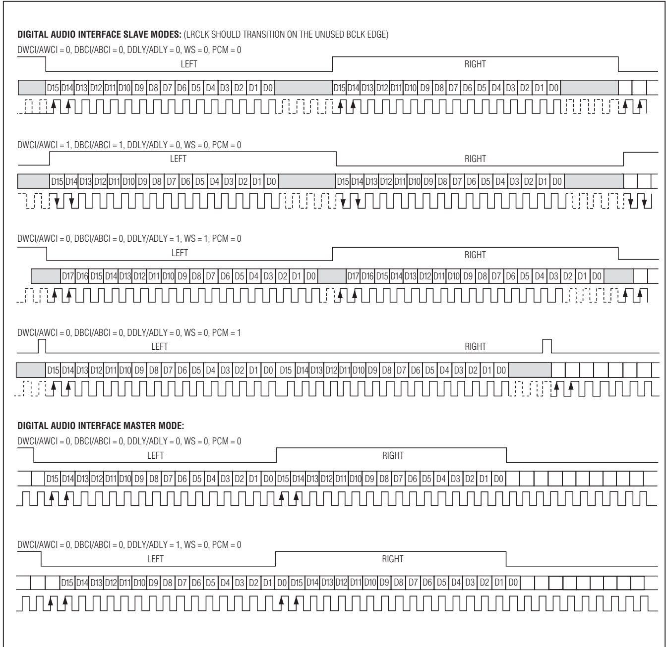
Figure 1. Digital Audio Interface Data Format Examples
