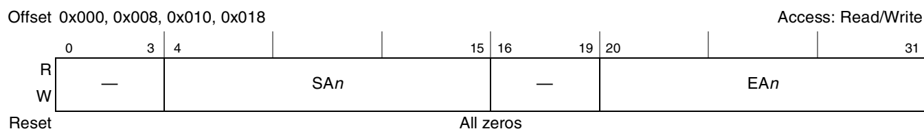
Figure 9-2. Chip Select Bounds Registers ( CS_n\_BNDS )
