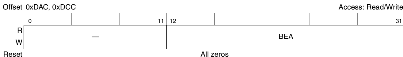
Figure 17-13. PCI Inbound Window Base Extended Address Registers (PIWBEAR n )
