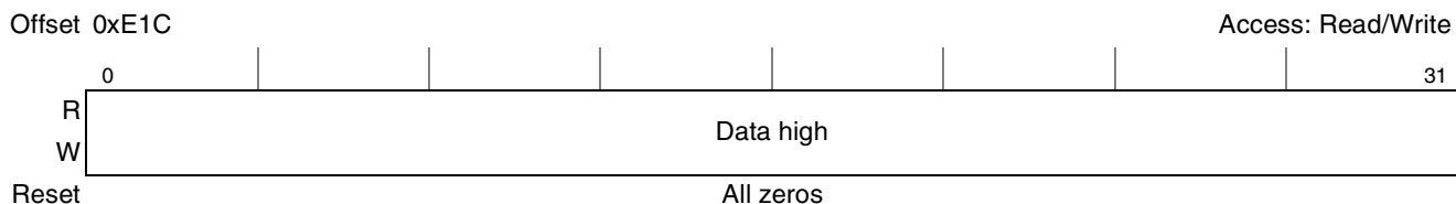
Figure 17-22. PCI Error Data High Capture Register (ERR_DH)
