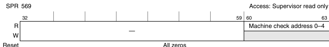
Figure 6-26. Machine Check Address Register Upper (MCARU)
