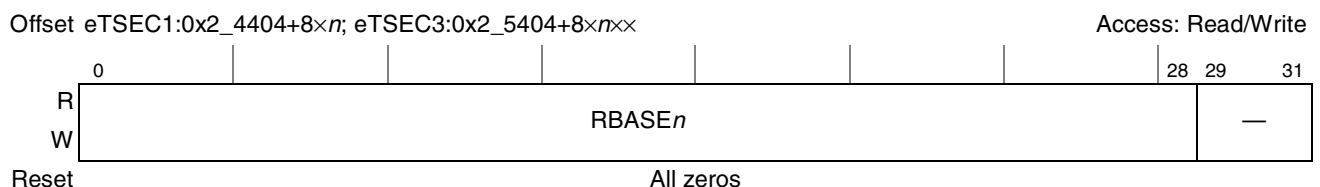
Figure 15-35. RBASE Register Definition
