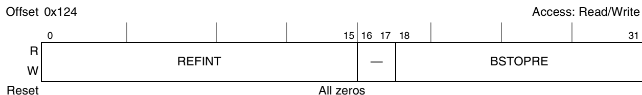
Figure 9-13. DDR SDRAM Interval Configuration Register (DDR_SDRAM_INTERVAL)
