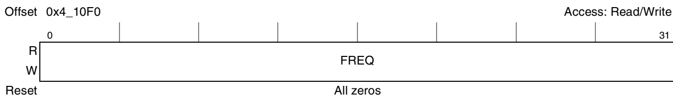
Figure 10-11. Timer Frequency Reporting Register (TFRR)
