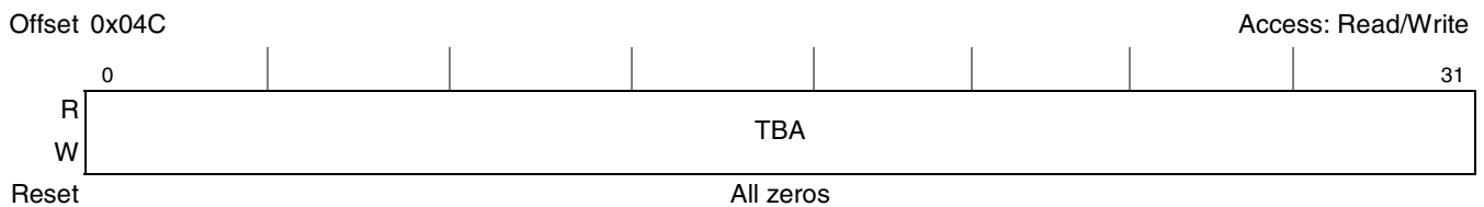
Figure 21-10. Trace Buffer Address Register (TBAR)
