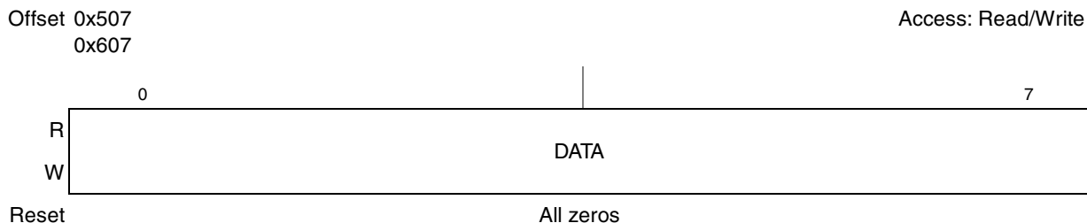
Figure 13-13. Scratch Register (USCR)
