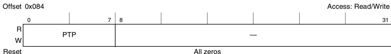
Figure 14-8. Memory Refresh Timer Prescaler Register (MRTPR)
