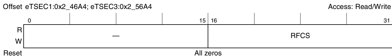
Figure 15-61. Receive FCS Error Counter Register Definition
