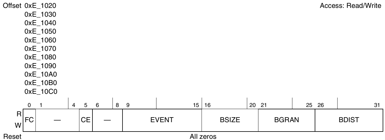
Figure 20-4. Performance Monitor Local Control A Registers (PMLCA1–PMLCA9)
