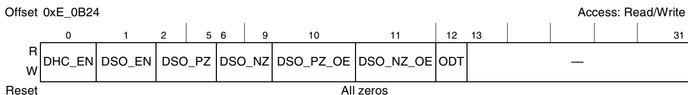
Figure 19-21. DDR Control Driver Register (DDRC DR)
