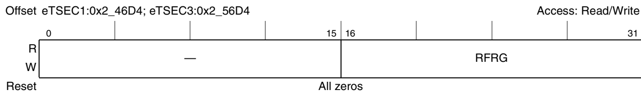
Figure 15-73. Receive Fragments Counter Register Definition
