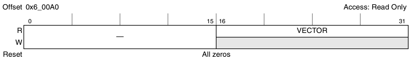
Figure 10-46. Processor Interrupt Acknowledge Register (IACK)
