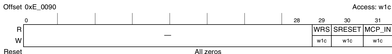
Figure 19-14. Machine Check Summary Register (MCPSUMR)
