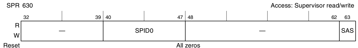
Figure 6-48. MAS Register 6 (MAS6)
