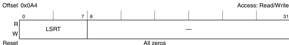
Figure 14-12. LSRT SDRAM Refresh Timer (LSRT)
