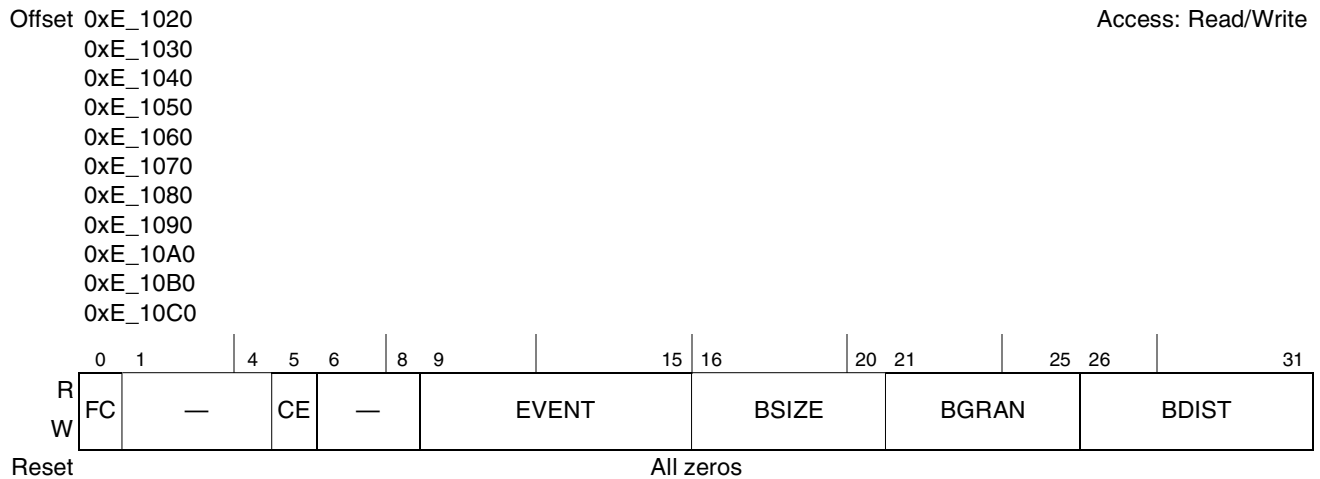
Figure 20-4. Performance Monitor Local Control A Registers (PMLCA1–PMLCA9)
