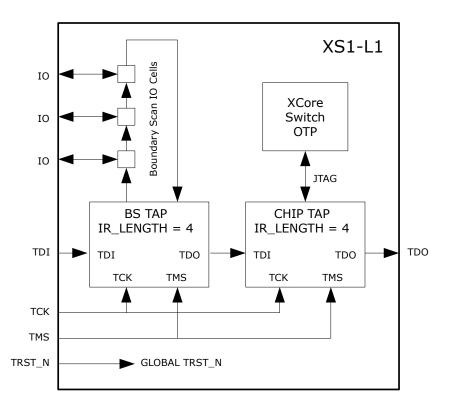
A diagram of the JTAG chain structure is shown below:
