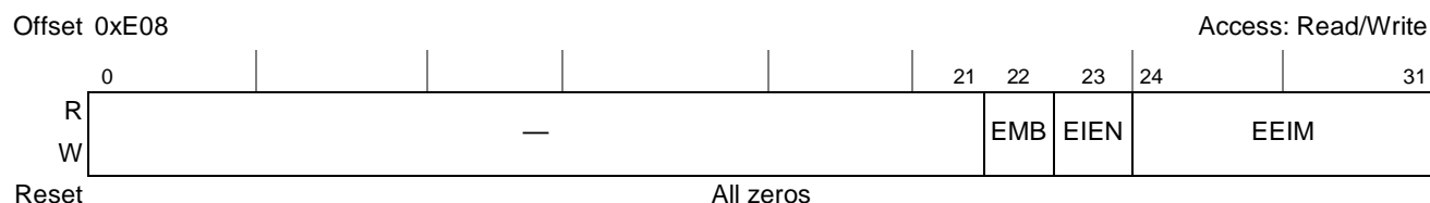
Figure 9-21. Memory Data Path Error Injection Mask ECC Register (ERR_INJECT)
