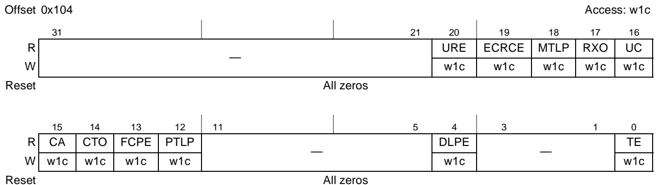
Figure 14-67. PCI Express Uncorrectable Error Status Register
