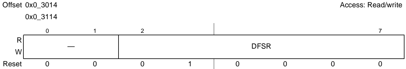
Figure 17-7. I 2 C Digital Filter Sampling Rate Register (I2CDFSRR)
