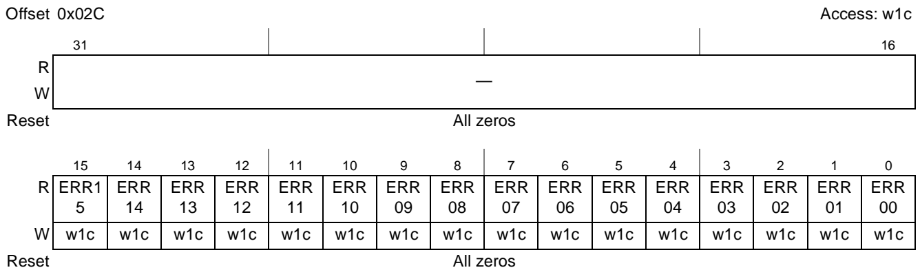
Figure 12-12. DMA Error Register (DMAERR)
