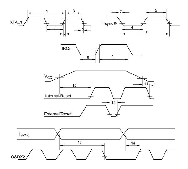
Figure 22 Timing Requirements of External Inputs
