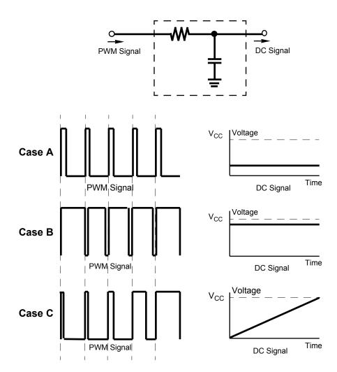
Figure 20 Analog Signals Generated from PWM Signals
