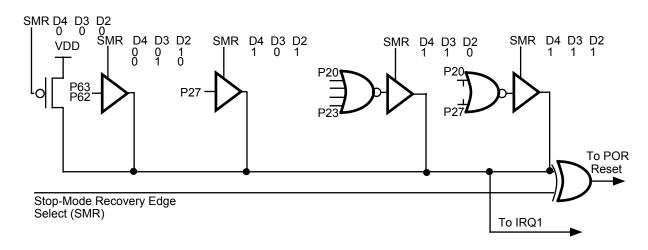
Figure 7 **Stop Mode Recovery Source/Level Select**
