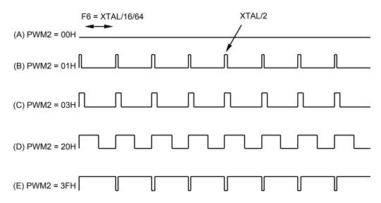
Figure 18 Pulse Width Modulator Timing Diagram, 6 Bit
