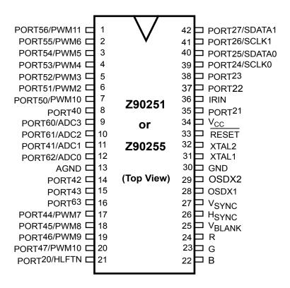
Figure 3 Z90255 and Z90251 Pin Assignments
