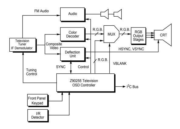
Figure 1 Z90255-Based TV System Application
