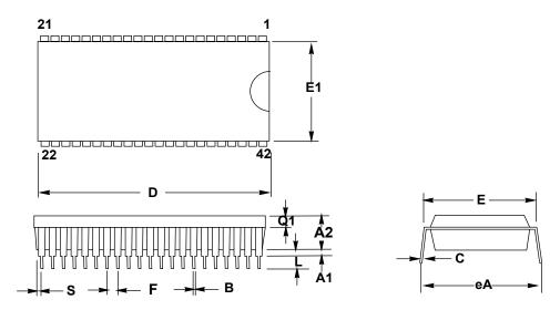
Figure 23 42-Lead Shrink Dual-in-line Package (SDIP)
