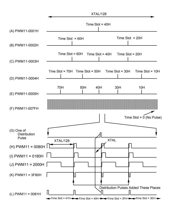
Figure 19 Pulse Width Modulator Timing Diagram, 14-Bit
