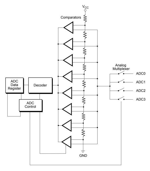
Figure 21 ADC Block Diagram
