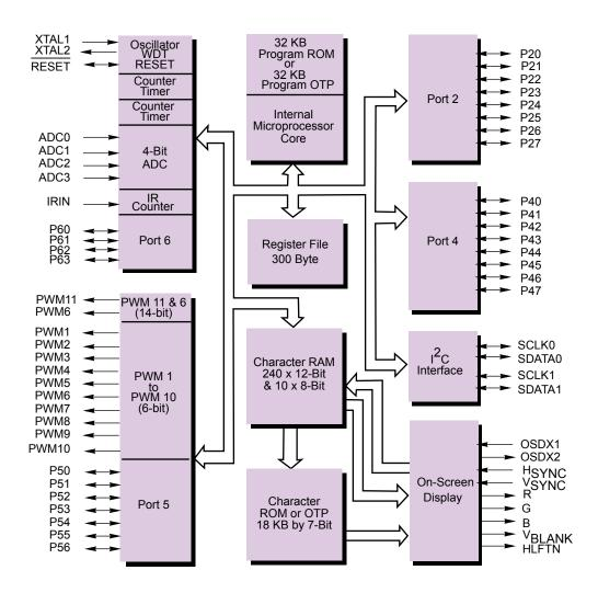
Figure 2 Z90255 Block Diagram
