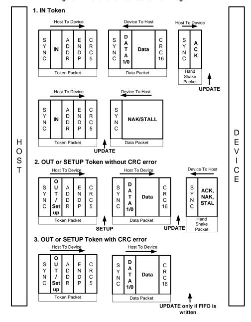
Figure 47. Token and Data Packet Flow Diagram
