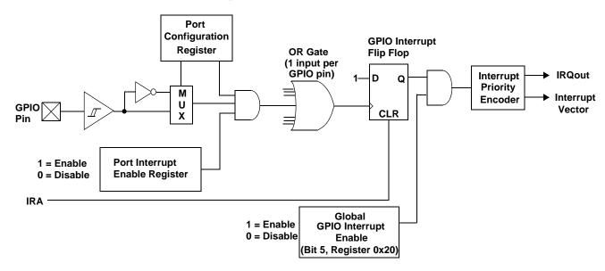
If one port pin has triggered an interrupt, no other port pins cause a GPIO interrupt until that port pin has returned to its inactive (non trigger) state or its corresponding port interrupt enable bit is cleared. The USB Controller does not assign interrupt priority to different port pins and the Port Interrupt Enable Registers are not cleared during the interrupt acknowledge process.
