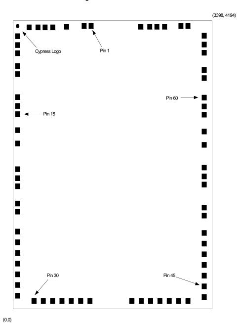
DIE STEP: 3398 x 4194 microns Die Size: 3322 x 4129 microns Die Thickness: 14 mils = 355.6 microns Pad Size: 80 x 80 microns
