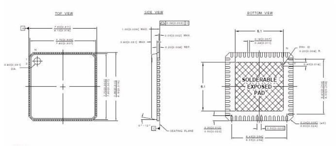
Figure 55. 56-Pin QFN 8 x 8 MM LF56A
