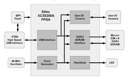
It contains a USB interface block, a User I/O block, a DDR2 SDRAM interface, a Heartbeat pulse generator, and a clock generator. The SPI Flash is used to store the design's FPGA configuration file.
