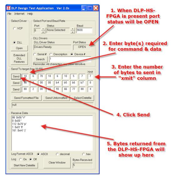
The commands used to interface to the DLP-HS-FPGA are detailed in Section 10 of this datasheet.
