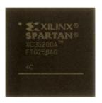
The FPGA device used on the DLP-HS-FPGA is the Xilinx Spartan™ 3A: XC3S200A-4FTG256
