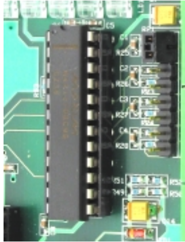
Figure 4: Oblique view of the 4-20mA Shunt Locations
