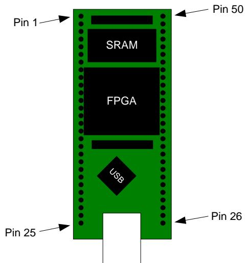
Top View (Interface Headers on bottom of PCB)
