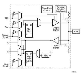
Figure 5. XC4000 and XC4000A Families Input/Output Block
