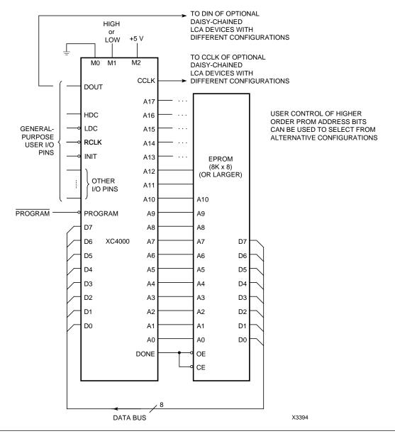
In Master Parallel mode, the lead LCA device directly addresses an industry-standard byte-wide EPROM, and accepts eight data bits right before incrementing (or decrementing) the address outputs.
