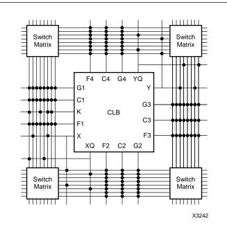
Figure 6. Typical CLB Connections to Adjacent Single-Length Lines
