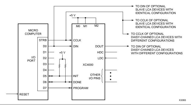
In Slave Serial mode, an external signal drives the CCLK input(s) of the LCA device(s). The serial configuration bitstream must be available at the DIN input of the lead LCA device a short set-up time before each rising CCLK edge. The lead LCA device then presents the preamble data (and all data that overflows the lead device) on its DOUT pin.
