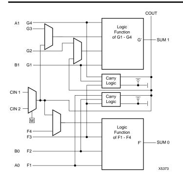
Figure 2. Fast Carry Logic in Each CLB
