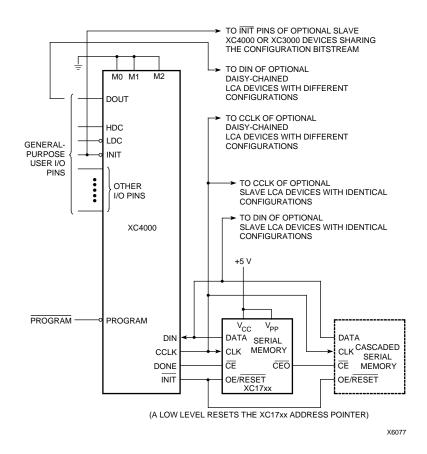
In Master Serial mode, the CCLK output of the lead LCA device drives a Xilinx Serial PROM that feeds the LCA DIN input. Each rising edge of the CCLK output increments the Serial PROM internal address counter. This puts the next data bit on the SPROM data output, connected to the LCA DIN pin. The lead LCA device accepts this data on the subsequent rising CCLK edge.
