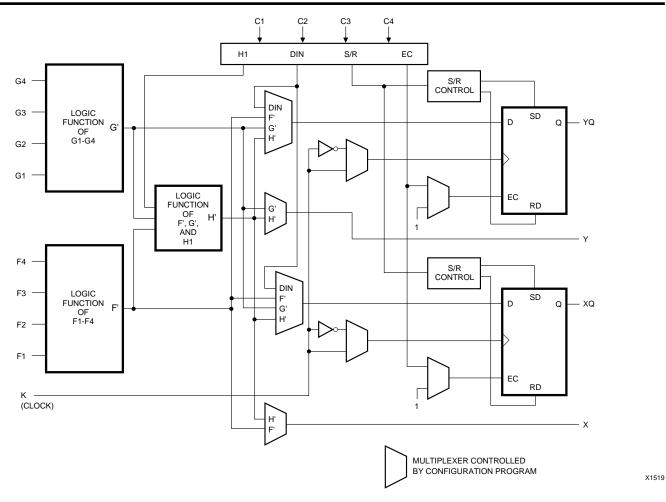
Figure 13. Simplified Block Diagram of XC4000 Configurable Logic Block
