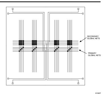
Figure 17. XC4000 Global Net Distribution. Four Lines per Column; Eight Inputs in the Four Chip Corners.
