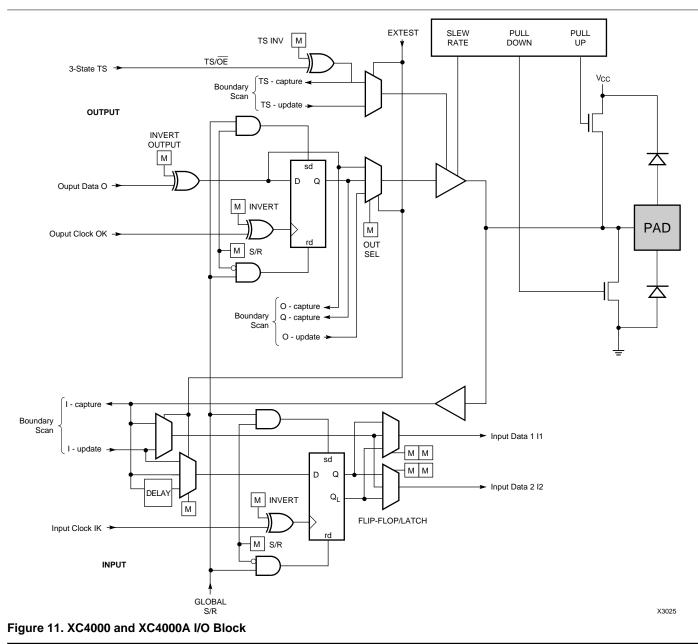
The inputs drive TTL-compatible buffers with 1.2-V input threshold and a slight hysteresis of about 300 mV. These buffers drive the internal logic as well as the D-input of the input flip-flop.
