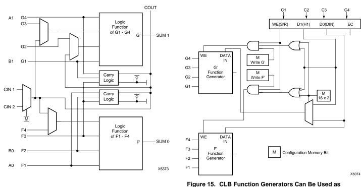
Figure 14. Fast Carry Logic in Each CLB
