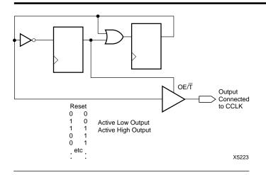
the extra CCLK pulse. This solution requires one CLB, one IOB and pin, and an internal oscillator with a frequency of up to 5 MHz as available clock source. Obviously, this XC3000 master device must be configured with late Internal Reset, which happens to be the default option.
