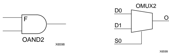
Figure 21: Output AND and MUX Symbols in XC4000EX IOB
