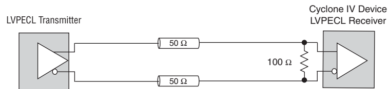
Figure 6-19. LVPECL DC-Coupled Termination ( Note 1 )
