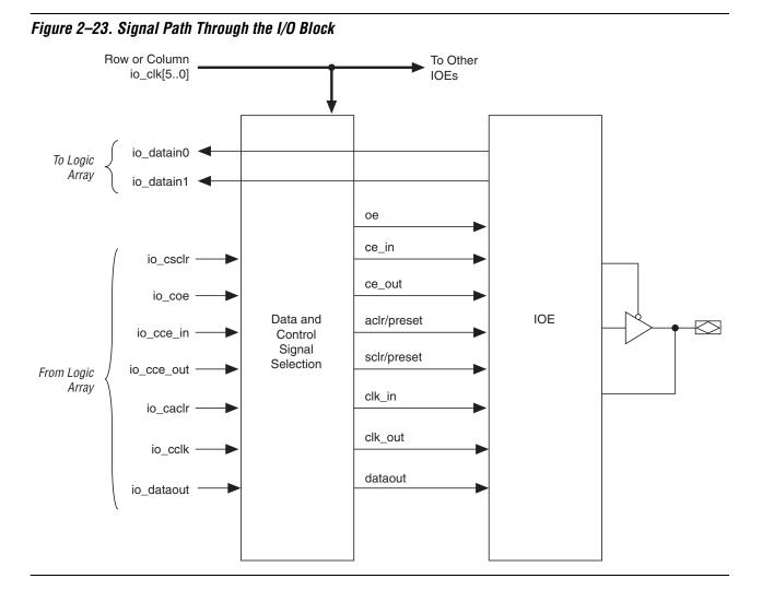
Each IOE contains its own control signal selection for the following control signals: oe, ce\_in, ce\_out, aclr/preset, sclr/preset, clk\_in, and clk\_out. Figure 2–24 illustrates the control signal selection.
