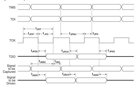
Figure 5–7. Cyclone II JTAG Waveform
