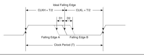
DCD expressed in absolution derivation, for example, D1 or D2 in Figure 5–8, is clock-period independent. DCD can also be expressed as a percentage, and the percentage number is clock-period dependent. DCD as a percentage is defined as:
