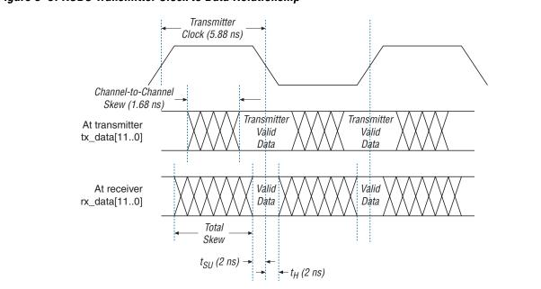
Table 5–49 shows the mini-LVDS transmitter timing budget for Cyclone II devices at 311 Mbps. Cyclone II devices cannot receive mini-LVDS data because the devices are intended for applications where they will be driving display drivers. A maximum mini-LVDS data rate of 311 Mbps is supported for Cyclone II devices using DDIO registers. Cyclone II devices support mini-LVDS only in the commercial temperature range.
