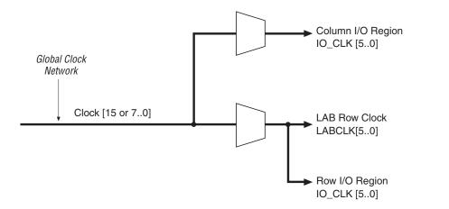
LAB row clocks can feed LEs, M4K memory blocks, and embedded multipliers. The LAB row clocks also extend to the row I/O clock regions.
