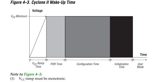
The  $V_{CC}$  ramp time and POR time will depend on the device characteristics and the power supply used in your system. The fast-on devices require a maximum  $V_{CC}$  ramp time of 2 ms and have a maximum POR time of 12 ms.
