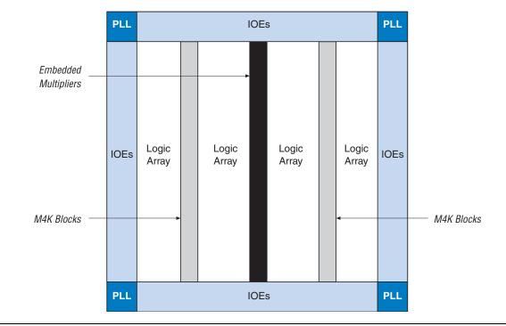
The number of M4K memory blocks, embedded multiplier blocks, PLLs, rows, and columns vary per device.
