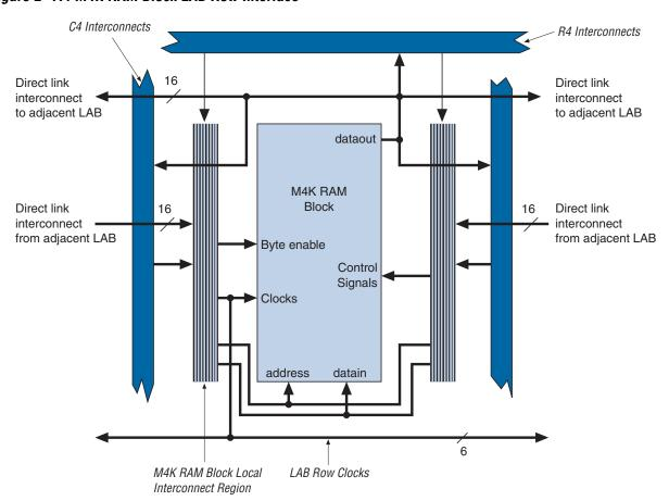
Figure 2–17. M4K RAM Block LAB Row Interface
