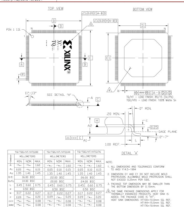
JEDEC MS-026-BFB REF. JEDEC W2-056-BED JEDEC MS-026-BGA THE SMALLEST CIRCLE AS PIN-1 I.D. 100, 144, and 176-PIN TQFP (TQ100/TQG100, TQ144/TQG144, and TQ176/TQG176)
