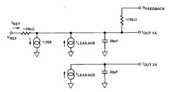
Figure 3. Equivalent DAC Circuit (All Digital Inputs HIGH)
