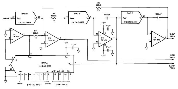
Figure 9. A Digitally Programmable Universal Active Filter
