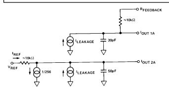
Figure 4. Equivalent DAC Circuit (All Digital Inputs LOW)
