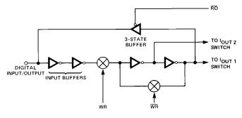
Figure 5. Digital Input/Output Structure
