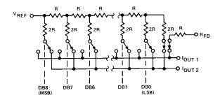
Figure 1. Simplified D/A Circuit of DAC8408
