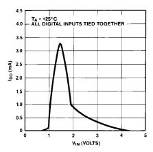
Supply Current vs. Logic Level
