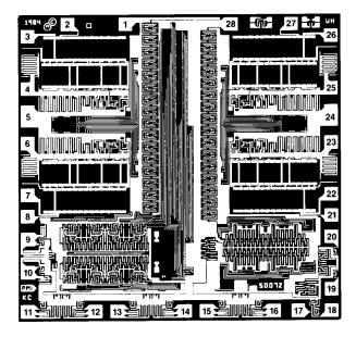
DIE SIZE  $0.130 \times 0.124$  inch, 16,120 sq. mils  $(3.30 \times 3.15 \text{ mm}, 10.4 \text{ sq. mm})$
