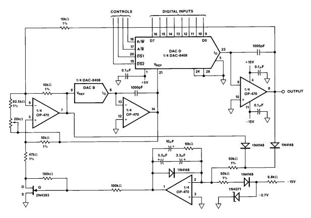
Figure 11. A Digitally Programmable, Low-Distortion Sinewave Oscillator
