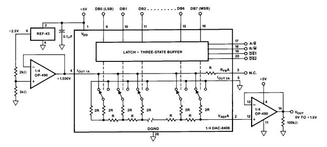
Figure 8. Unipolar Supply, Voltage Output DAC Operation
