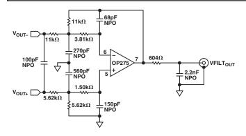
Figure 13. Suggested Output Filter Schematic
