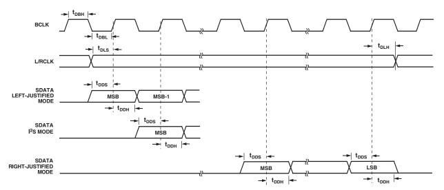
Figure 3. Serial Port Timing
