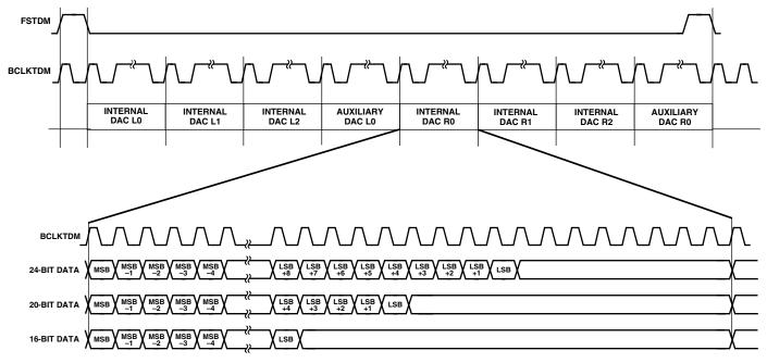
Figure 9. TDM Mode Timing
