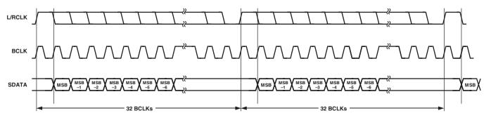
Figure 10. DSP Mode Timing
