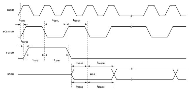
Figure 4. TDM Master and Slave Mode Timing
