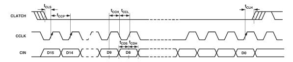
Figure 2. SPI Port Timing
