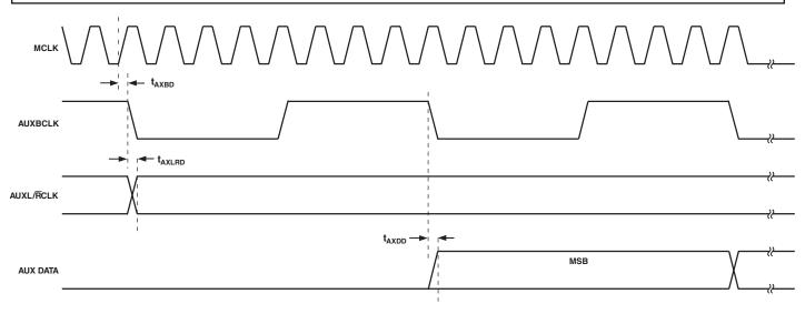
Figure 5. Auxiliary Interface Timing
