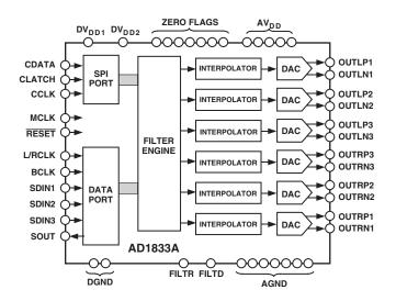
The AD1833A is fully compatible with all known DVD formats, accommodating word lengths of up to 24 bits at sample rates of 48 kHz and 96 kHz on all six channels while supporting a 192 kHz sample rate on two channels. It also provides the Redbook standard 50  $\mu$ s/15  $\mu$ s digital de-emphasis filters at sample rates of 32 kHz, 44.1 kHz, and 48 kHz.
