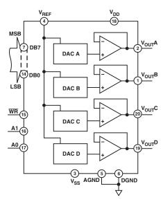
Figure 8. AD7226 Unipolar Output Circuit
