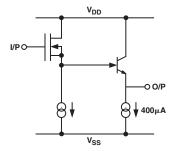
Figure 2. Amplifier Output Stage
