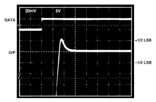
Figure 7a. Positive Step Settling Time ( $V_{SS} = -5 V$ )
