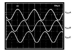
Figure 13. 3-Phase Sine Wave Output
