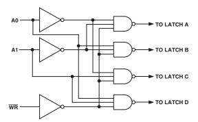
Figure 4. Input Control Logic
