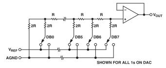
Figure 1. D/A Simplified Circuit Diagram
