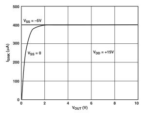
Figure 3. Variation of  $I_{SINK}$  with  $V_{OUT}$
