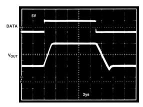
Figure 6. Dynamic Response ( $V_{SS} = -5 V$ )
