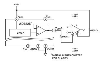
Figure 17. Offset Adjust for AD544
