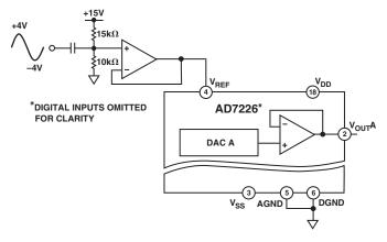
Figure 16. Varying Reference Signal
