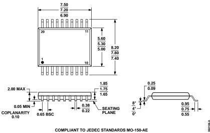
Figure 3. 20-Lead Shrink Small Outline Package [SSOP] (RS-20) Dimensions shown in millimeters
