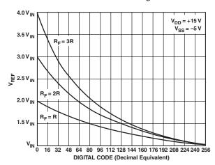
Figure 12. Variation of  $V_{REF}$  with Feedback Configuration
