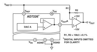
Figure 9. AD7226 Bipolar Output Circuit
