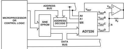
Figure 11. 3-Phase Sine Wave Generation Circuit
