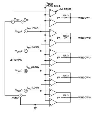
Figure 14a. Logic Level Measurement
