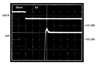
Figure 7b. Negative Step Settling Time ( $V_{SS} = -5 V$ )
