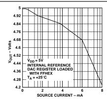
Figure 3. Output Source Current Capability with  $V_{DD} = 5 V$
