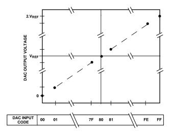
Figure 26. DAC Transfer Function
