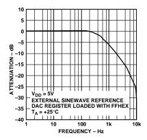
Figure 8. Large Scale Signal Frequency Response
