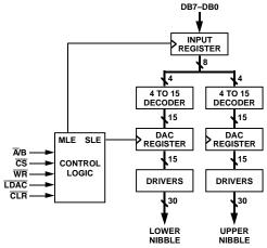
Figure 22. Register Arrangement
