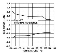
Figure 16. Typical DNL vs. Temperature
