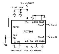
Figure 27. Typical Configuration Selecting the Internal Reference
