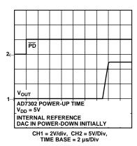
Figure 10. Exiting Power-Down (Full Power-Down)
