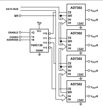
Figure 33. Decoding Multiple AD7302 DACs in a System
