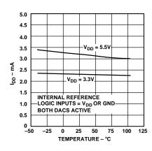
Figure 6. Typical Supply Current vs. Temperature
