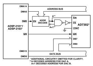
Figure 29. AD7302-ADSP-2101/ADSP-2103 Interface
