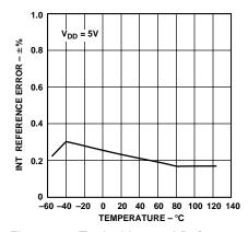
Figure 17. Typical Internal Reference Error vs. Temperature
