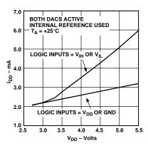
Figure 7. Typical Supply Current vs. Supply Voltage
