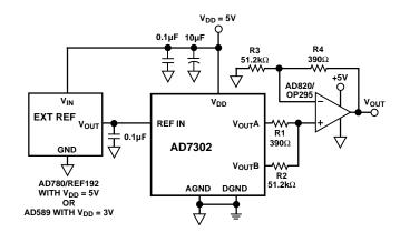
Figure 36. Coarse/Fine Adjust Circuit
