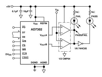
Figure 34. Programmable Window Detector
