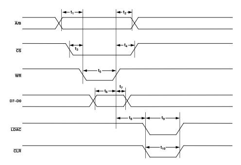
Figure 1. Timing Diagram for Parallel Data Write
