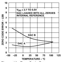
Figure 12. Zero Code Error vs. Temperature
