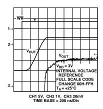
Figure 9. Full-Scale Settling Time
