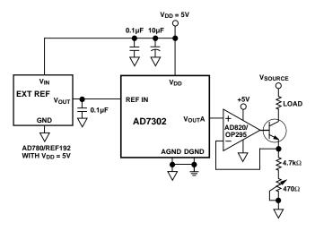
Figure 35. Programmable Current Source
