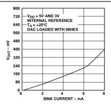
Figure 2. Output Sink Current Capability with  $V_{DD} = 3 V$  and  $V_{DD} = 5 V$
