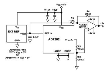
Figure 32. Bipolar Operation Using the AD7302
