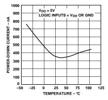
Figure 18. Power-Down Current vs. Temperature
