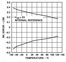
Figure 15. Typical INL vs. Temperature
