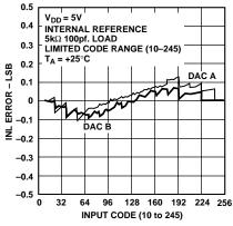
Figure 14. Integral Linearity Plot
