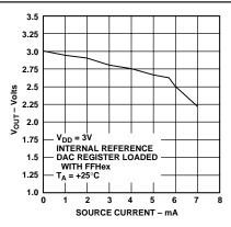
Figure 4. Output Source Current Capability with  $V_{DD} = 3 V$
