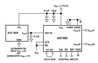
Figure 28. Typical Configuration Using An External Reference
