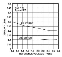
Figure 5. Relative Accuracy vs. External Reference
