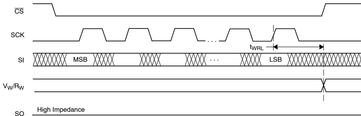
Figure 6. Potentiometer Timing (for All Load Instructions)
