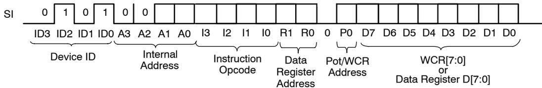
Figure 8. Three-Byte Instruction Sequence
