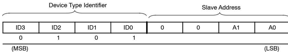
Figure 4. Identification Byte Format 0101 Device Type Identifier (MSB)
