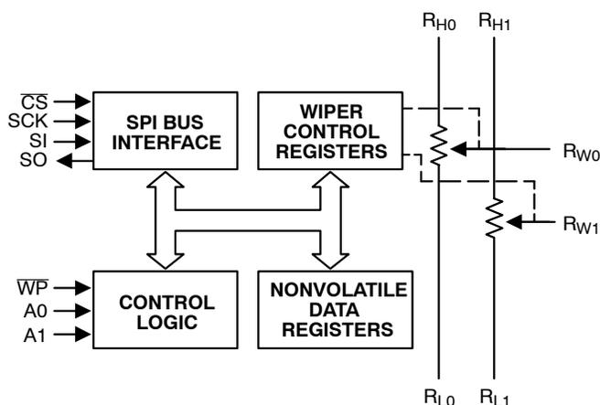
Figure 1. Functional Diagram
