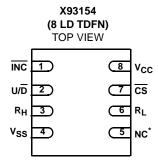
$^{\rm NC}$  can be left unconnected, or connected to any voltage between  $\rm V_{SS}$  and  $\rm V_{CC}$
