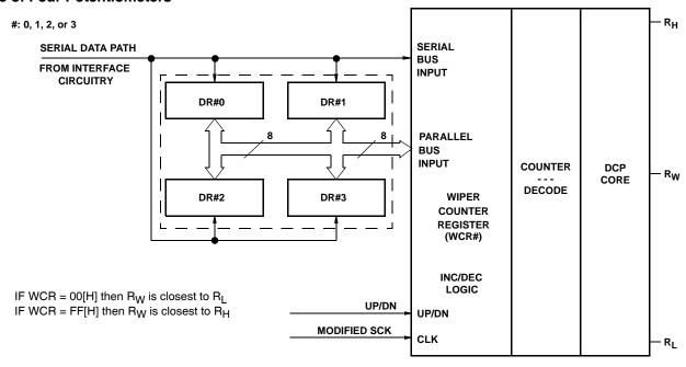
FIGURE 1. DETAILED POTENTIOMETER BLOCK DIAGRAM
