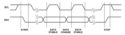
FIGURE 2. VALID DATA CHANGES, START, AND STOP CONDITIONS
