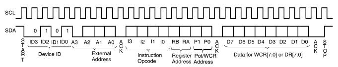
FIGURE 5. THREE-BYTE INSTRUCTION SEQUENCE 2-WIRE INTERFACE
