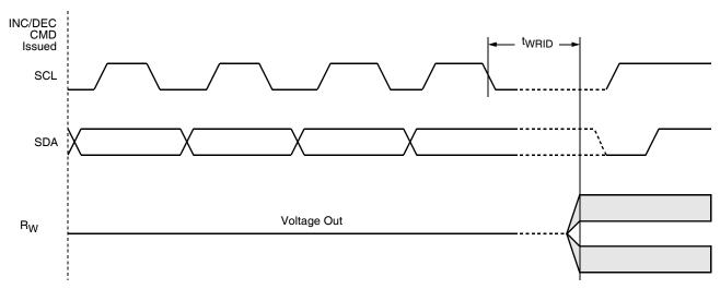
FIGURE 7. INCREMENT/DECREMENT TIMING SPEC
