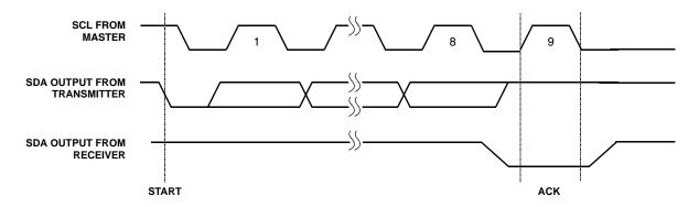
FIGURE 3. ACKNOWLEDGE RESPONSE FROM RECEIVER
