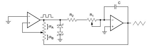
$frequency \propto R_1,\,R_2,\,C$ amplitude  $\propto R_A$ ,  $R_B$
