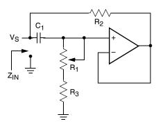
$$Z_{IN} = R_2 + s R_2 (R_1 + R_3) C_1 = R_2 + s Leq$$
