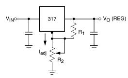
$V_O (REG) = 1.25V (1+R_2/R_1)+I_{adj} R_2$
