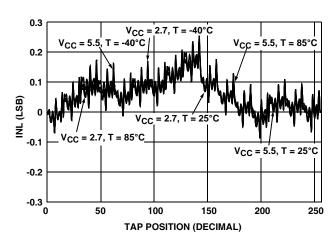
FIGURE 4. INL vs TAP POSITION IN VOLTAGE DIVIDER MODE FOR  $10k\Omega$  (W)
