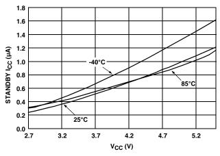
FIGURE 2. STANDBY  $I_{CC}$  vs  $V_{CC}$
