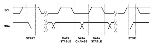
FIGURE 15. VALID DATA CHANGES, START, AND STOP CONDITIONS
