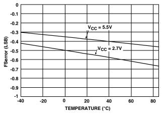
FIGURE 6. FSerror vs TEMPERATURE
