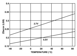
FIGURE 5. ZSerror vs TEMPERATURE
