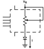
TWO-TERMINAL VARIABLE RESISTOR; VARIABLE CURRENT
