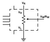
THREE-TERMINAL POTENTIOMETER; VARIABLE VOLTAGE DIVIDER
