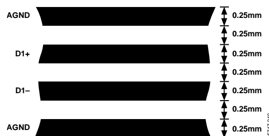
Figure 61. Arrangement of Signal Tracks
