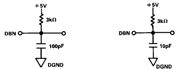
Figure 5. Load Circuit for \overline{INT} Propagation Delays
