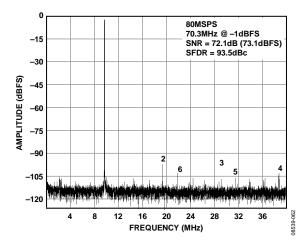
Figure 5. AD9649-80 Single-Tone FFT with  $f_{IN} = 70.3 \text{ MHz}$
