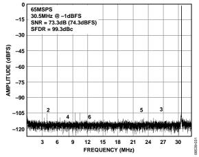
Figure 18. AD9649-65 Single-Tone FFT with  $f_{IN} = 30.5$  MHz
