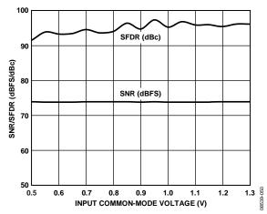
Figure 37. SNR/SFDR vs. Input Common-Mode Voltage,  $f_{IN} = 10.3 \text{ MHz}, f_S = 20 \text{ MSPS}$
