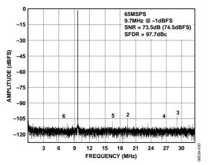
Figure 16. AD9649-65 Single-Tone FFT with  $f_{IN} = 9.7 \text{ MHz}$
