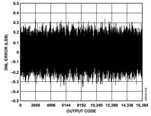
Figure 12. AD9649-80 DNL Error with  $f_{IN} = 9.7$  MHz
