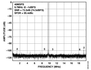
Figure 21. AD9649-40 Single-Tone FFT with  $f_{IN} = 9.7 \text{ MHz}$
