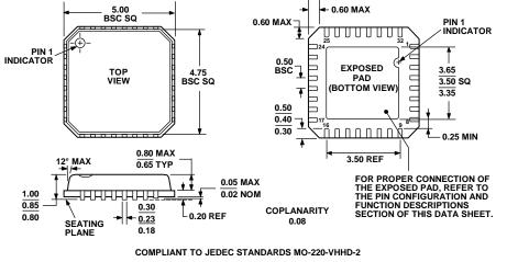
Figure 56. 32-Lead Lead Frame Chip Scale Package [LFCSP\_VQ] 5 mm × 5 mm Body, Very Thin Quad (CP-32-4)
