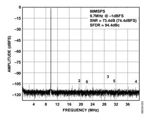
Figure 4. AD9649-80 Single-Tone FFT with  $f_{IN} = 9.7$  MHz
