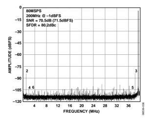
Figure 8. AD9649-80 Single-Tone FFT with  $f_{IN} = 200 \text{ MHz}$
