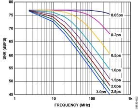
Figure 53. SNR vs. Input Frequency and Jitter
