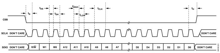
Figure 55. Serial Port Interface Timing Diagram
