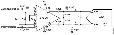
Figure 42. Differential Input Configuration Using the AD8352
