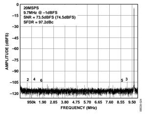
Figure 24. AD9649-20 Single-Tone FFT with  $f_{IN} = 9.7 \text{ MHz}$
