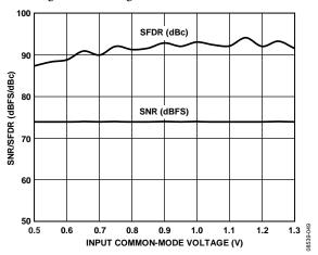
Figure 36. SNR/SFDR vs. Input Common-Mode Voltage,  $f_{IN} = 32.1 \text{ MHz}, f_S = 80 \text{ MSPS}$
