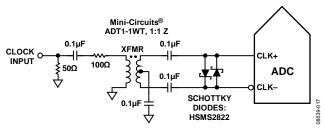
Figure 47. Transformer-Coupled Differential Clock (3 MHz to 200 MHz)
