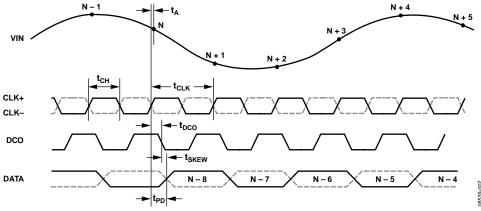
Figure 2. CMOS Output Data Timing
