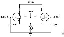
Figure 46. Equivalent Clock Input Circuit
