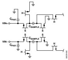
Figure 35. Switched-Capacitor Input Circuit
