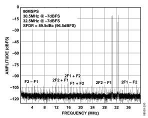
Figure 6. AD9649-80 Two-Tone FFT with  $f_{\text{IN1}} = 30.5$  MHz and  $f_{\text{IN2}} = 32.5$  MHz
