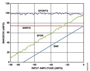
Figure 23. AD9649-40 SNR/SFDR vs. Input Amplitude (AIN) with  $f_{\rm IN} = 9.7$  MHz
