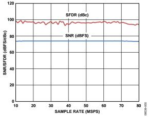
Figure 11. AD9649-80 SNR/SFDR vs. Sample Rate with AIN =  $9.7 \, \text{MHz}$
