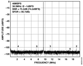
Figure 22. AD9649-40 Single-Tone FFT with  $f_{IN} = 30.5$  MHz
