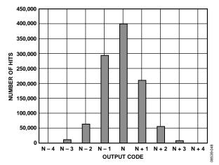
Figure 14. AD9649-80 Grounded Input Histogram
