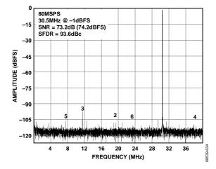
Figure 7. AD9649-80 Single-Tone FFT with  $f_{IN} = 30.5 \text{ MHz}$
