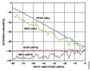
Figure 9. AD9649-80 Two-Tone SFDR/IMD3 vs. Input Amplitude (AIN) with  $f_{\rm IN1}=30.5$  MHz and  $f_{\rm IN2}=32.5$  MHz
