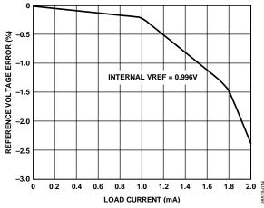
Figure 44. VREF Accuracy vs. Load Current
