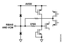
Figure 34. Equivalent RBIAS, VCM Circuit
