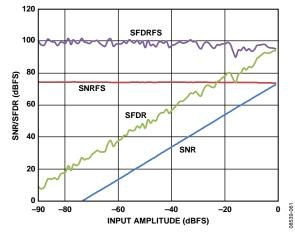
Figure 13. AD9649-80 SNR/SFDR vs. Input Amplitude (AIN) with  $f_{\rm IN}=9.7~\rm MHz$
