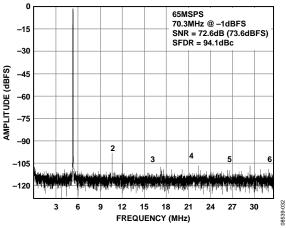
Figure 17. AD9649-65 Single-Tone FFT with  $f_{IN} = 70.3$  MHz
