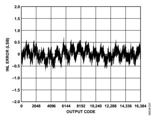
Figure 15. AD9649-80 INL with  $f_{IN} = 9.7 \text{ MHz}$
