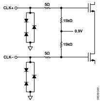
Figure 30. Equivalent Clock Input Circuit
