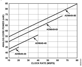
Figure 54. Analog Core Power vs. Clock Rate
