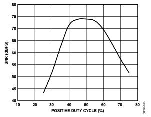
Figure 52. SNR vs. Clock Duty Cycle
