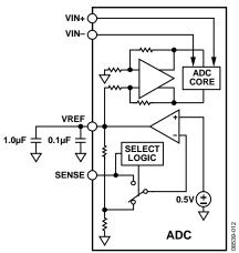
Figure 43. Internal Reference Configuration
