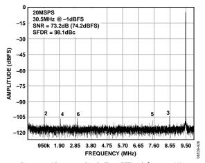
Figure 25. AD9649-20 Single-Tone FFT with  $f_{\rm IN}$  = 30.5 MHz
