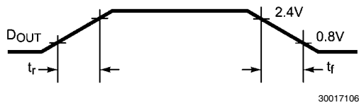
FIGURE 4. D OUT Rise and Fall Times
