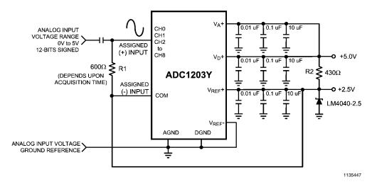
FIGURE 12. Pseudo-Differential Biasing with the Signal Source AC Coupled Directly into the ADC
