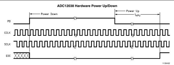
Note: Hardware power up/down may occur at any time. If PD is high while a conversion is in progress that conversion will be corrupted and erroneous data will be stored in the output shift register.
