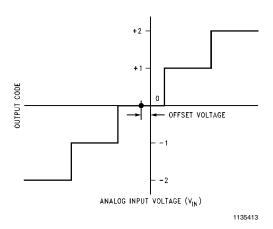
FIGURE 4. Offset or Zero Error Voltage
