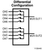
A/DIN1 and A/DIN2 can be assigned as the + or - input
