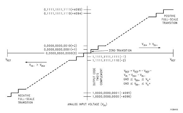
FIGURE 1. Transfer Characteristic
