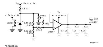
FIGURE 16. Low Drift Extremely Stable Reference Circuit
