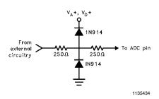
FIGURE 6. Protecting the MUXOUT1, MUXOUT2, A/DIN1 and A/DIN2 Analog Pins
