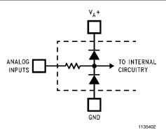
Note 8: To guarantee accuracy, it is required that the  $V_A$ + and  $V_D$ + be connected together to the same power supply with separate bypass capacitors at each V+ pin.
