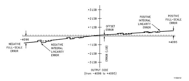
FIGURE 3. Simplified Error Curve vs. Output Code after Auto Calibration Cycle
