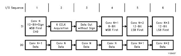
FIGURE 8. Changing the ADC's Conversion Configuration
