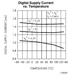
**Typical Dynamic Performance Characteristics** The following curves apply for 12-bit + sign mode after Auto Calibration unless otherwise specified.
