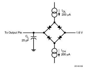
FIGURE 1. Timing Test Circuit
