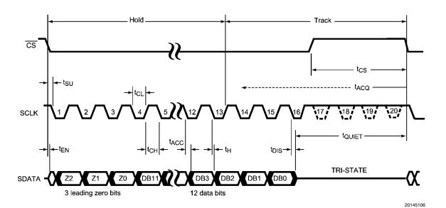
FIGURE 2. ADC121S021 Serial Timing Diagram
