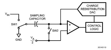
FIGURE 4. ADC121S021 in Hold Mode
