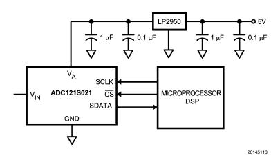
**FIGURE 6. Typical Application Circuit**
