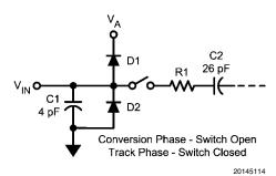
FIGURE 7. Equivalent Input Circuit
