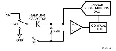
FIGURE 3. ADC121S021 in Track Mode
