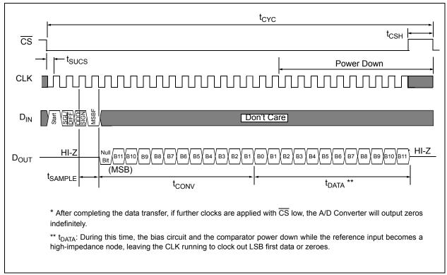
FIGURE 5-2: Communication with MCP3202 using LSB first format.
