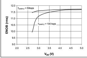
**FIGURE 2-25:** Effective Number of Bits (ENOB) vs. V<sub>DD</sub>.
