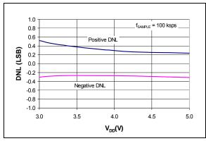
FIGURE 2-9: (DNL) vs. V<sub>DD</sub>.
