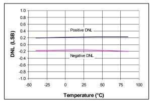
FIGURE 2-14: Differential Nonlinearity (DNL) vs. Temperature.
