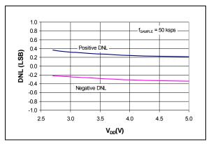
FIGURE 2-12: Differential Nonlinearity (DNL) vs. V<sub>DD</sub>.
