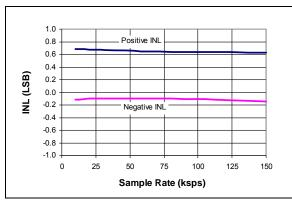
FIGURE 2-1:Integral Nonlinearity (INL)vs. Sample Rate.
