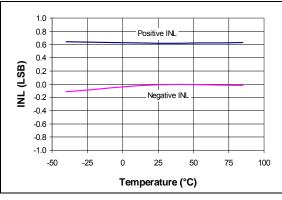
FIGURE 2-7: Integral Nonlinearity (INL) vs. Temperature.
