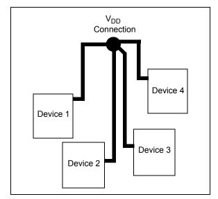
*FIGURE 6-4:* V<sub>DD</sub> traces arranged in a 'Star' configuration in order to reduce errors caused by current return paths.
