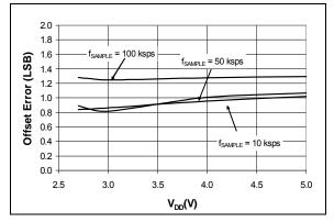
FIGURE 2-18: Offset Error vs. V<sub>DD</sub>.
