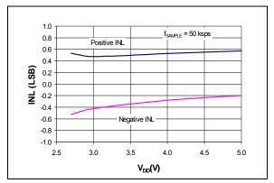
FIGURE 2-5: Integral Nonlinearity (INL) vs. V<sub>DD</sub>.
