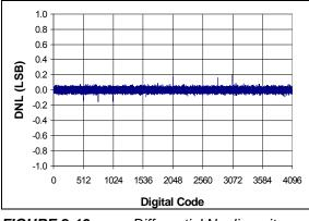
FIGURE 2-13: Differential Nonlinearity (DNL) vs. Code (Representative Part).
