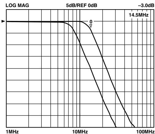
TPC 23. Rx LPF Frequency Response, Low f_c , 0 \times 60 and 0 \times 96 Tuning Targets
