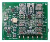
The MCP651 Input Offset Evaluation board is intended to provide a simple means to measure the MCP651 Input Offset Evaluation Board op amp's input offset voltage under a variety of operating conditions. The measured input offset voltage (VOST) includes the input offset voltage specified in the data sheet (VOS) plus changes due to: power supply voltage (PSRR), common mode voltage (CMRR), output voltage (AOL), input offset voltage drift over temperature ( $\Delta$ VOS/ $\Delta$ T) and 1/f noise.
