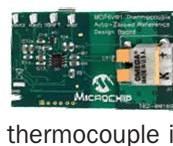
The MCP6V01 design board demonstrates how to use a difference amplifier system to measure Electromotive Force (EMF) voltage at the cold junction of thermocouple in order to accurately measure temperature of the thermocouple bead. This can be done by using the MCP6V01 auto-zeroed op amp because of its ultra low offset Voltage (VOS) and high Common Mode Rejection Ratio (CMRR).
