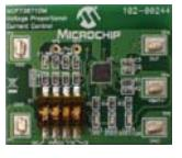
The MCP73871 Demo Board with Voltage Proportional Current Control is designed to demonstrate Microchip's stand-alone linear Li-Ion battery charger with system power path and load sharing management control solution. The MCP73871 integrates the required elements to meet design challenges when developing new Li-Ion/Li-Polymer batteries powered products.
