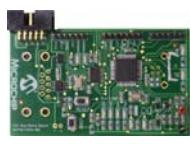
The MCP2515 CAN Bus Monitor Demo board kit contains two identical boards which can be connected together to create a simple two node Controller Area Network (CAN) bus, which can be controlled and/or monitored via the included PC interface. The board(s) can also be connected to an existing CAN bus.
