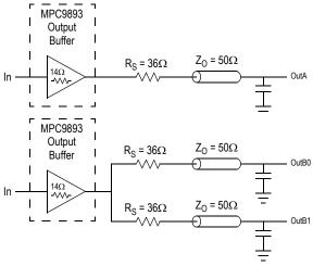
Figure 8. Single versus Dual Transmission Lines
