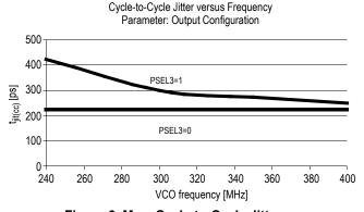
Figure 6. Max. Cycle-to-Cycle Jitter versus
