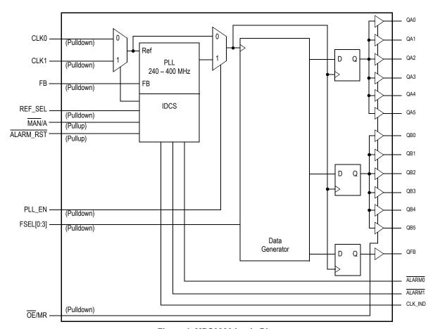
Figure 1. MPC9893 Logic Diagram
