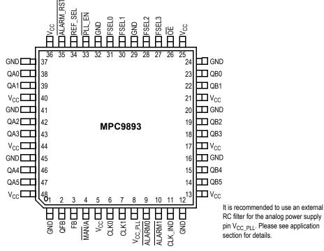
Figure 2. MPC9893 48-Lead Pinout (Top View)
