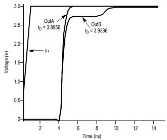
Figure 9. Single versus Dual Waveforms
