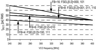
Figure 5. Max. I/O Phase Jitter versus VCO Frequency
