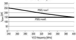
Figure 7. Max. Period Jitter versus VCO Frequency
