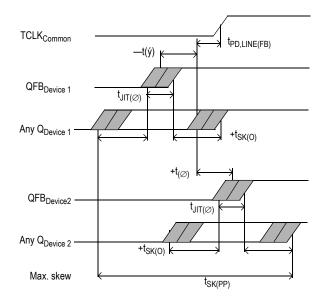
Figure 4. MPC9893 Max. Device-to-Device Skew
