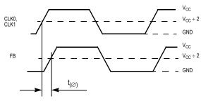
Figure 13. Propagation Delay  $(\mathbf{t}_{(\varnothing)},$  static phase offset) Test Reference
