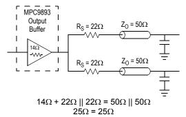
Figure 10. Optimized Dual Line Termination
