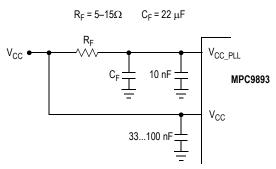
Figure 3. V<sub>CC PLL</sub> Power Supply Filter
