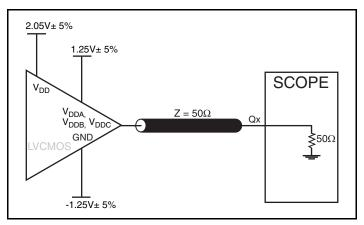
3.3V Core/2.5V Output Load AC Test Circuit
