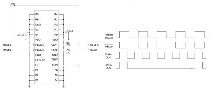
Note: The series termination resistor is located before the feedback trace.
