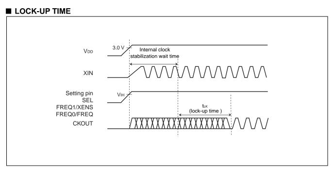
If the setting pin is fixed at the "H" or "L" level, the maximum time after the power is turned on until the set clock signal is output from CKOUT pin is (the stabilization wait time of input clock to XIN pin) + (the lock-up time "tLK"). For the input clock stabilization time, check the characteristics of the resonator or oscillator used.
