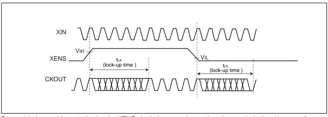
For modulation enable control using the XENS pin during normal operation, the set clock signal is output from CKOUT pin at most the lock-up time ( $t_{LK}$ ) after the level at the XENS pin is determined.
