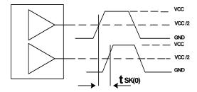
Figure 7. Output-to-Output Skew tsk(0)
