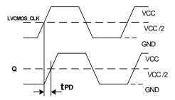
Figure 5. LVCMOS Propagation Delay (TPD) Test Reference
