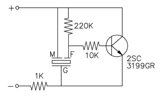
The current consumption and the sound pressure level are measured by using the recommended driving circuit shown above.
