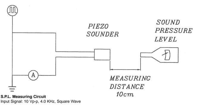
Mic: RION S.P.L. meter UC30 or equivalent S.G.: Hewlett Packard 33120A Function Generator or equivalent
