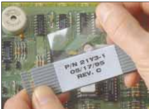
Flat Ribbon Cable Labeling
