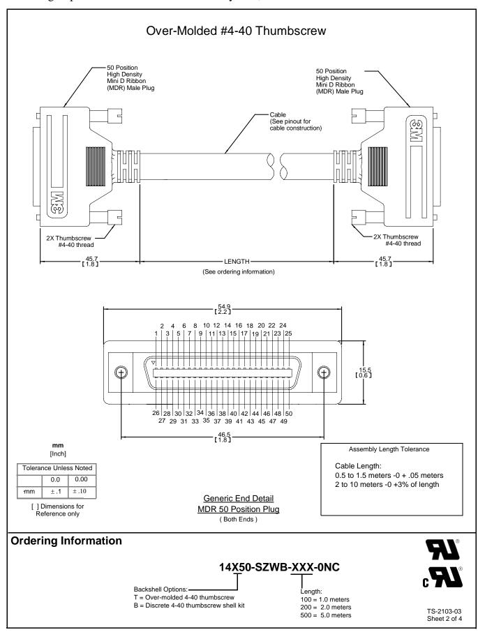
.050" High Speed Video Data Transmission System, 50 Position
